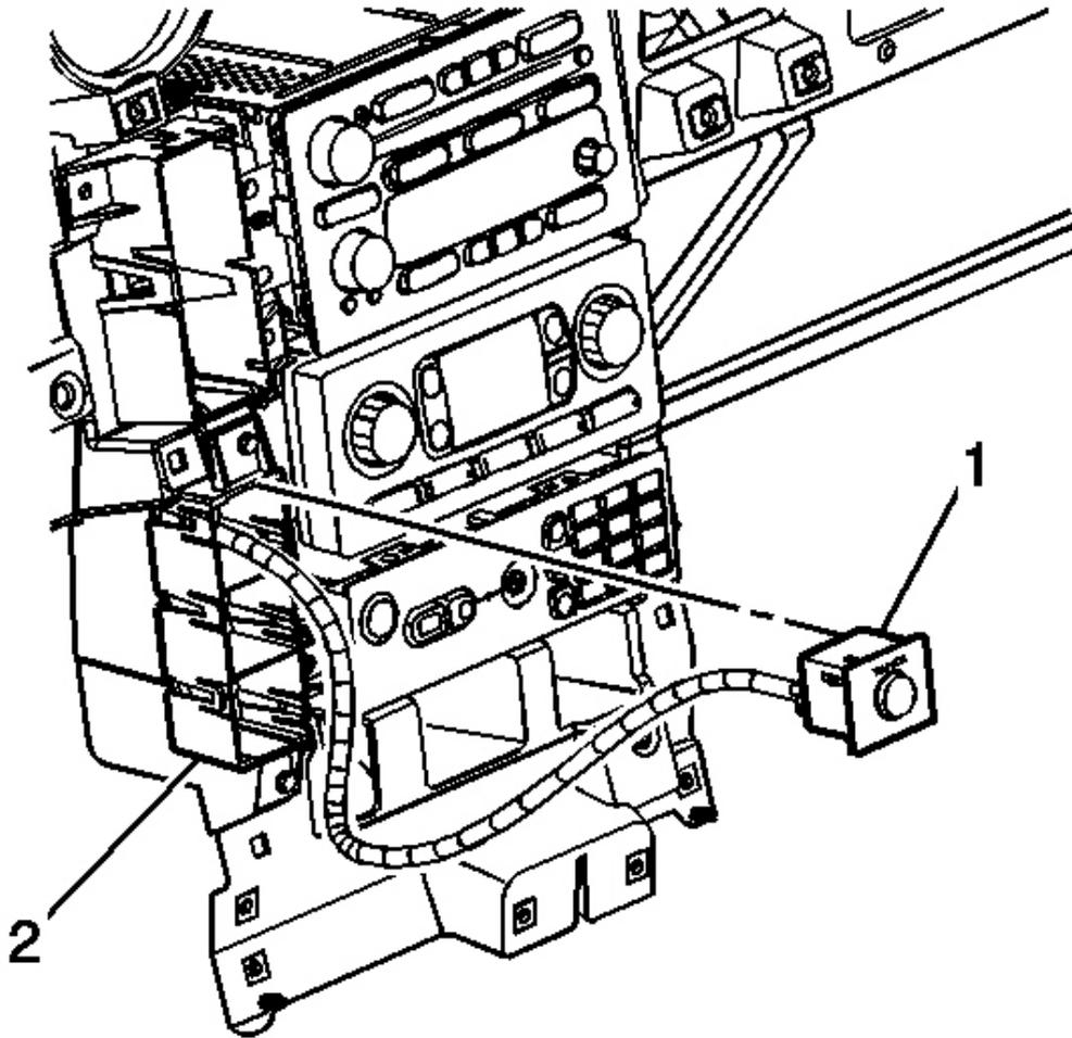
**Fig. 20: Traction Control Switch & I/P Assembly**
