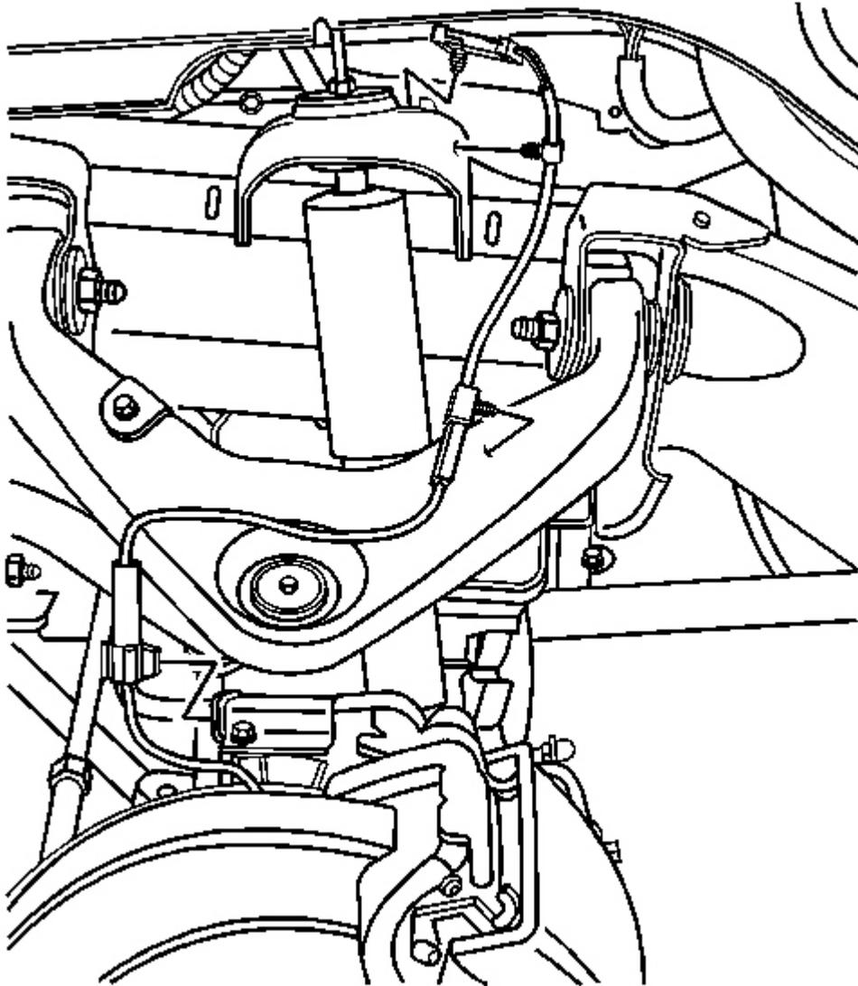
**Fig. 13: Front Wheel Speed Sensor Cable**
