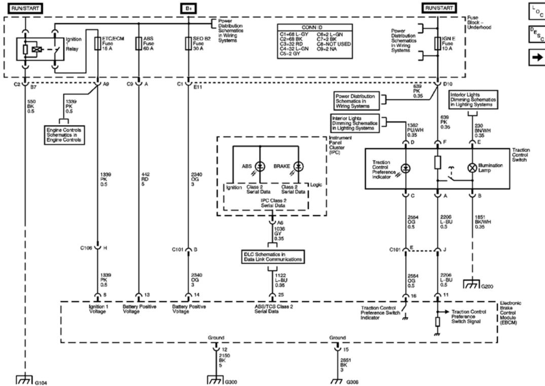
**Fig. 1: EBCM Power, Ground, DLC, Indicator Lamps, and Traction Control Switch**
