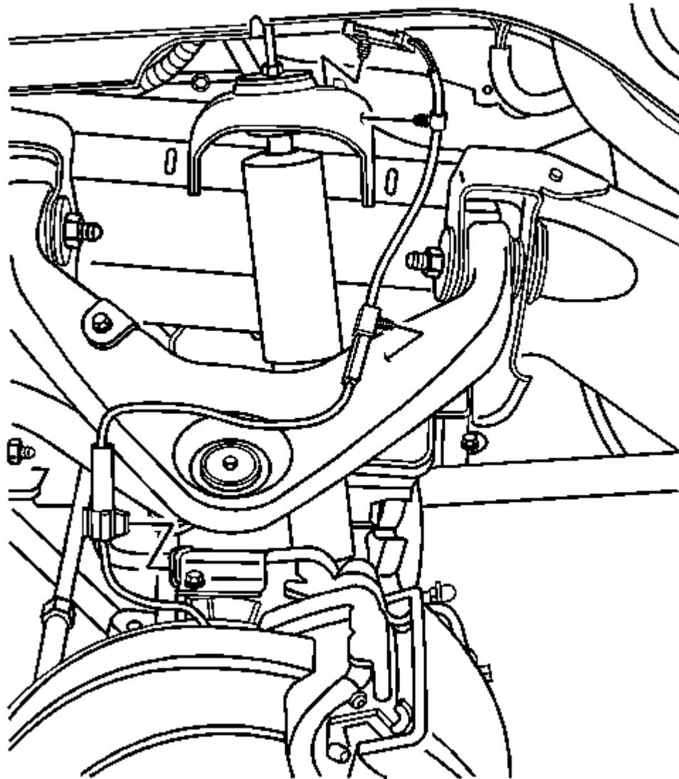
**Fig. 16: Front Wheel Speed Sensor Cable**
