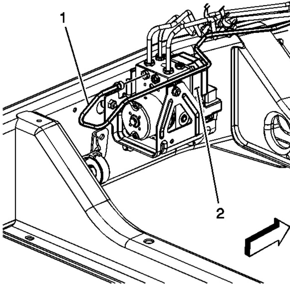
**Fig. 12: Right Front Brake Pipe & BPMV**
