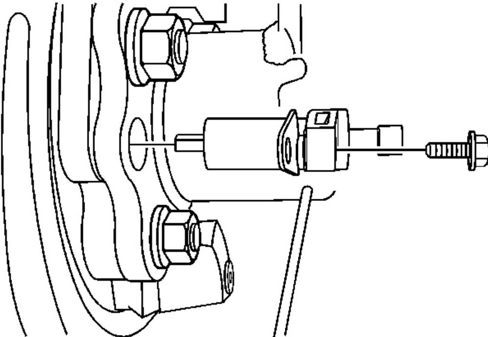
**Fig. 17: Rear Wheel Speed Sensor & Shim**
