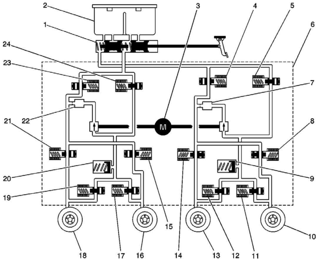
**Fig. 24: BPMV Hydraulic Flow**
