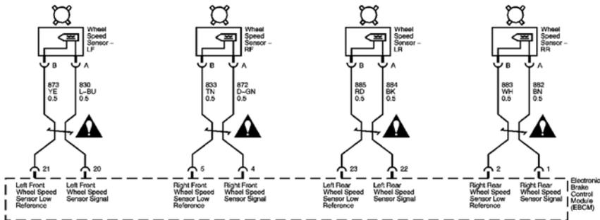
**Fig. 3: Wheel Speed Sensor Inputs**
