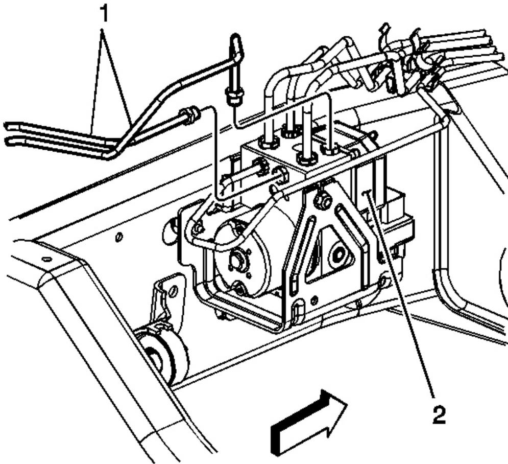
**Fig. 11: Rear Brake Pipes & BPMV**
