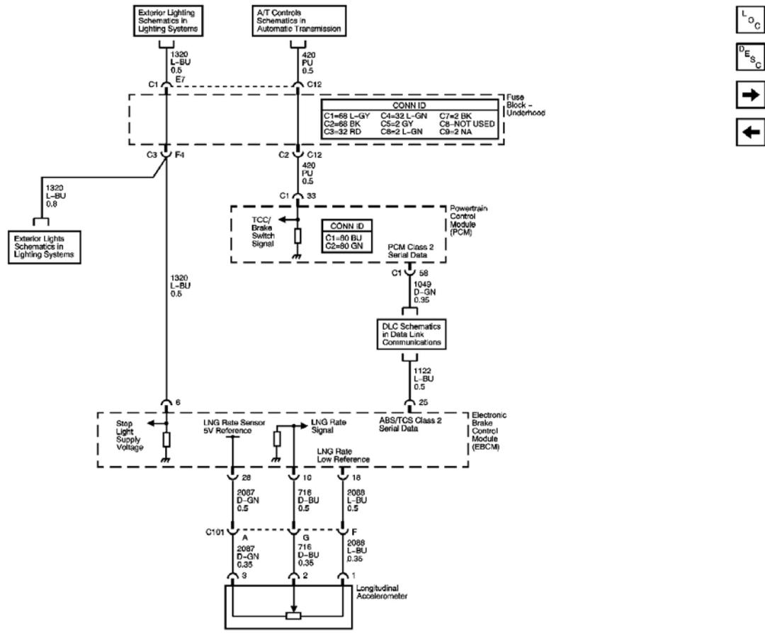
**Fig. 2: Stoplamp Switch and Longitudinal Accelerometer Inputs**
