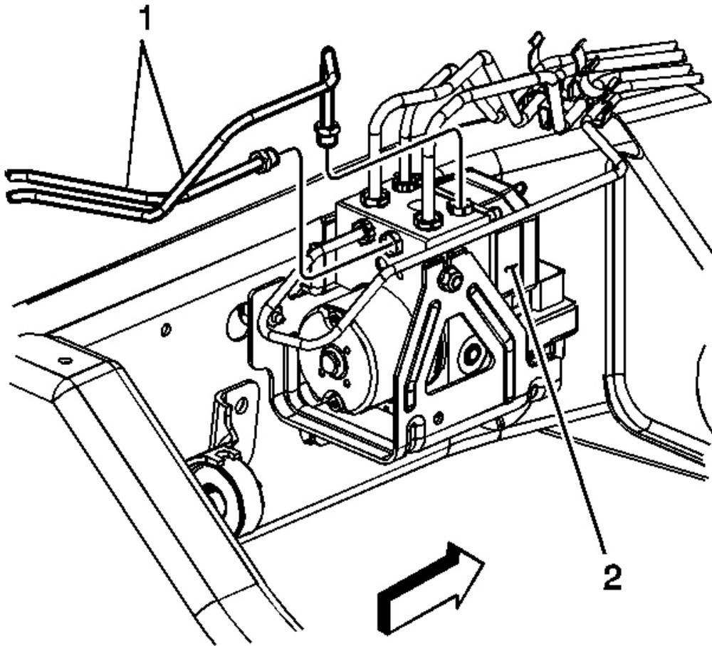
**Fig. 8: Rear Brake Pipes & BPMV**
